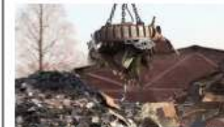
Ferrous metals are picked up by a giant magnet at a scrapyard
