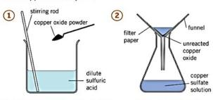
Add copper oxide powder (a base) to dilute sulfuric acid. Keep adding until some copper oxide is left over. All the acid has now reacted. Filter to remove the copper oxide that has not reacted.
