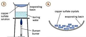
▲ Heat the copper sulfate solution in an evaporating basin until most of the water evaporates.
